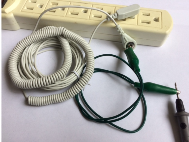
Figure 6: Setup with black meter lead, using an alligator clip cord, and Earthing grounding cord
