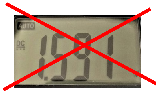
Figure 8. DO NOT SET THE DIAL TO DC!!!
