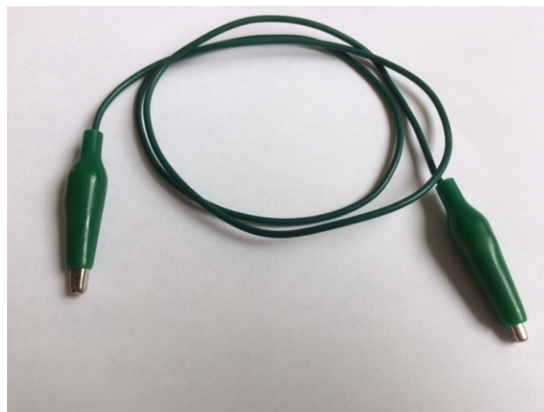
Figure 5: Cord with alligator clips on both ends
