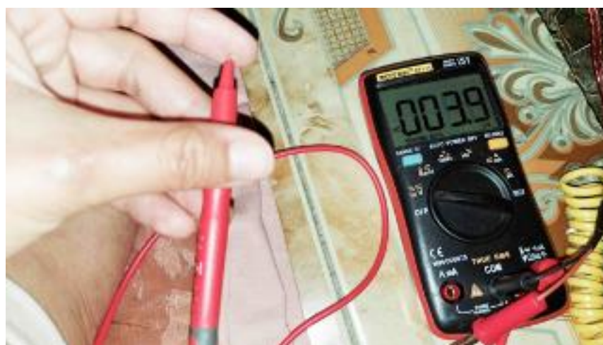
Figure 10. The result of reading the skin voltage after Earthing is 3.9 millivolts which means the tool is functioning optimally.
