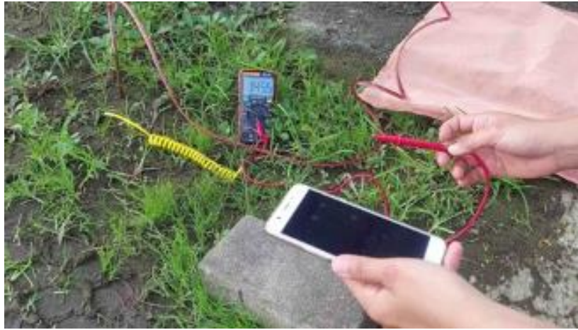
Figure 5. Trial of assembling the Earthing device stage 2, where the skin voltage when not touching the Earthing device reads 145.5 millivolts.
